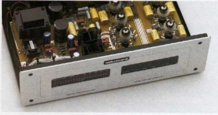
phono input to the main outputs is 54db. Although suitable for moving-magnet and high-output moving coil cartridges, it falls just short of providing the requisite oomph needed for low-output types. I used it with a high-output Grado, but added an Ortofon transformer to the mix when using the Linn LP12/Ekos/Arkiv combination.
